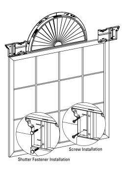
**Note:** The figures below show cross sections of the Header in place. In some instances the Header may rock on the high point of the siding. To overcome this problem, insert the screws or shutter fasteners into the wall evenly, working between top and bottom.
